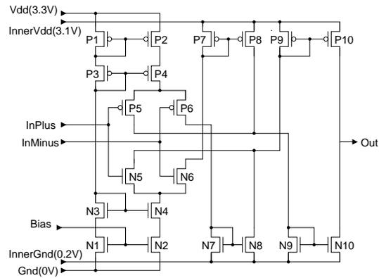
Figure 3: Amplifier topology. The input stage (P/N1-6) is cascoded (P/N3-4) to reduce offset, with the bias (N1-2) mirrored with pMOSFETs (P1-2) for rail-to-rail operation. The input stage operates between the outer power rails for maximal input range whereas the intermediate mirrors (P/N7-8) and output stage (P/N9-10) operate between the inner power rails as is the limitation for all signals which pass through the interconnect network.
