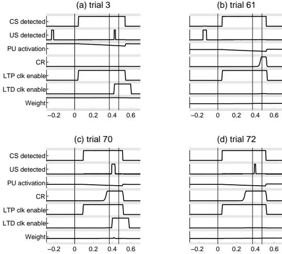
**Figure 5:** Results. Behaviour of chip signals during 4 example trials. Each graph shows the traces of 7 signals buffered out from the programmable core. Within each signal, the vertical scale shows the voltage range from 0 up to 3.3V. The number of the trial is given in the heading and time on the x-axis is relative to the CS onset, with three vertical lines marking, from left to right: CS onset, US onset and the offset of both stimuli.
