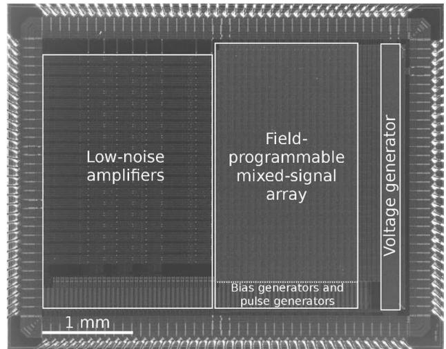
(a) The chip uses a  $0.35 \mu\text{m}$  process (Austria Microsystems), and has dimensions  $4.8 \times 3.8$  mm. Cores are indicated on the photo.
