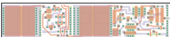
**TOP:** An 8-chip test set-up was used to create a grid of neurons. Each chip contains 32 integrated neuron circuits and each neuron had 64 dedicated circuits for incoming synapses.
